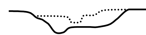
2020b Channel adjustment process is complete. Channel dimensions and relationship with flood plain are as they existed prior to channelization but at a lower elevation. Stable plan form (sinuosity) is restored but in a different location. Stable channel slope is achieved. Stream power is in balance with resistance of channel boundary materials and sediment transport needs.
